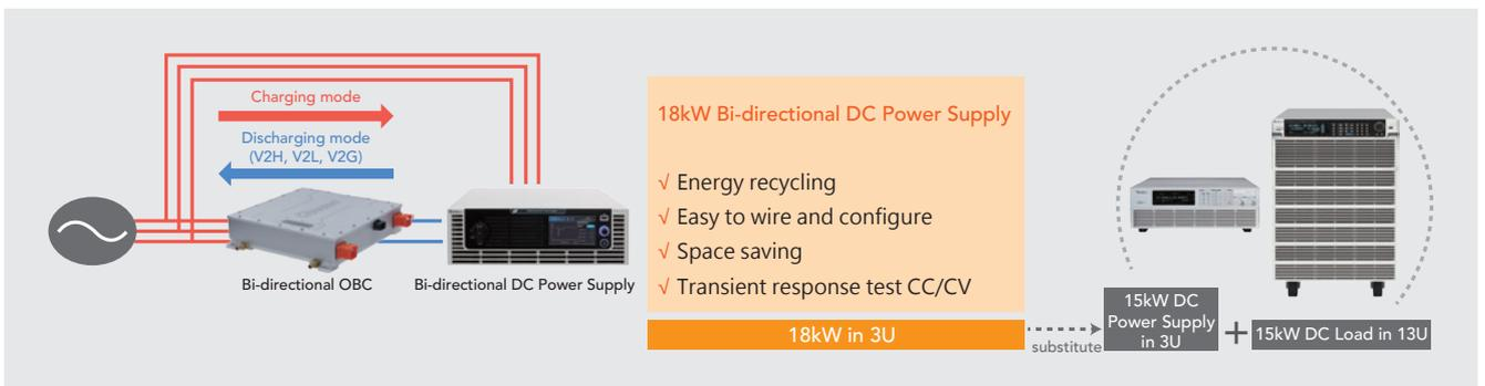
Bidirectional on-board charger testing configuration
