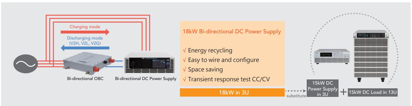
Bidirectional on-board charger testing configuration
